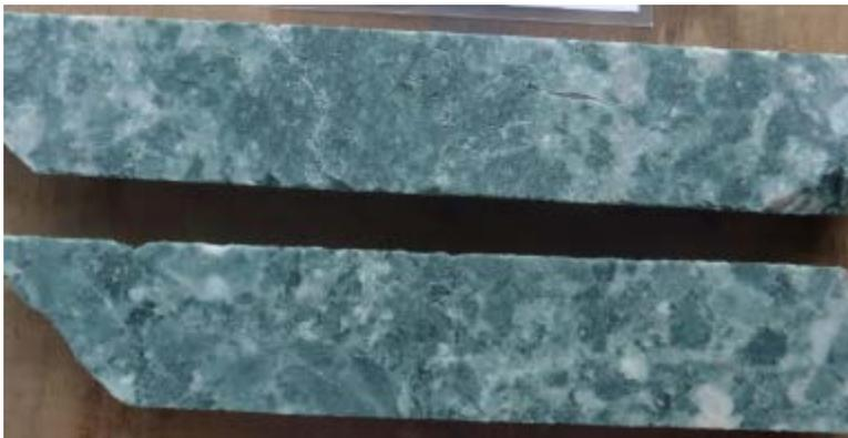
Photo 3. Weakly brecciated highly permeable dacite volcanics with strong chlorite-adularia-silica alteration from 899.85m in drill hole N62DDH015 (top) and 595m in drill hole N62DDH012 (bottom) (Harrington, 2015).
