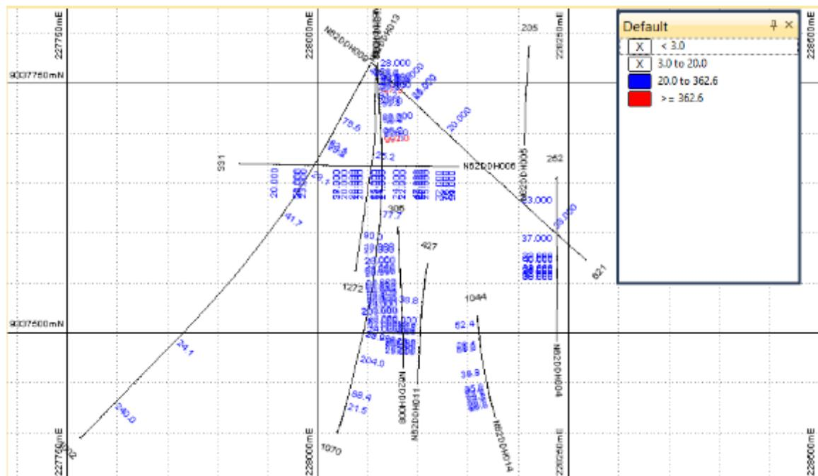
Figure 5. Drill hole Mo assays and XRF analysis (blue > 20-362ppm Mo, red >362ppm Mo) down-hole.
