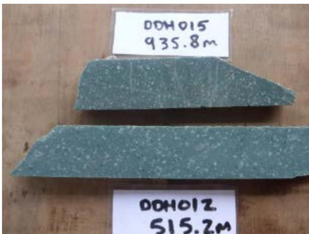
Photo 6. Diorite from 935.8m in drill hole DDH015 (top) and 515.2m in drill hole N62DDH012 (bottom) (Harrington, 2015).
