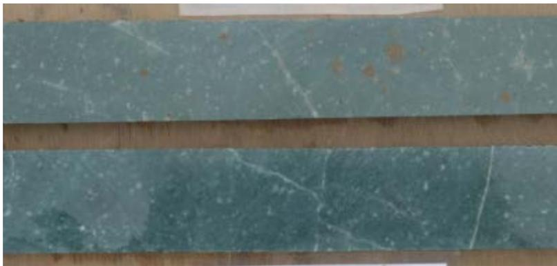
Photo 17. Diorite with disseminated pyrite and intense chlorite alteration from 975m in drill hole DDH012 (top) and from 925m in drill hole N62DDH015 (bottom) (Harrington, 2015).
