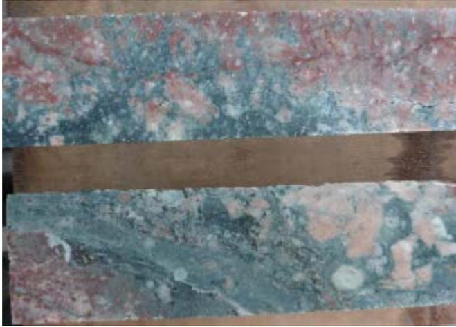
Photo 4. Chlorite-hematite-adularia (pink)-silica altered dacite volcanic with flattened pumice from 857.3m in drill hole N62DDH015 (top) and 564m in drill hole N62DDH012 (bottom) (Harrington, 2015).
