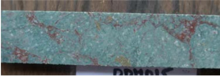
Photo 1. Chlorite-hematite  $\pm$  adularia altered dacite volcanic with disseminated pyrite from 838.m in drill hole N62DDH015 (Harrington, 2015).
