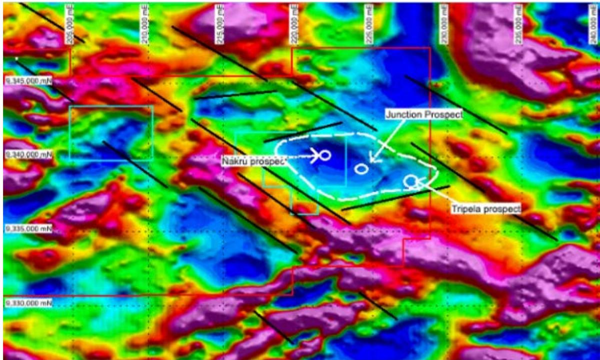
Figure 2. Reduced-to-Pole aeromagnetic data showing Cu-Au prospects within an interpreted fault jog developed during sinistral movement on the NW regional fractures, which facilitated the formation of a caldera with rim fractures (dotted white line) (from Menzies and Corbett, 2014). Orthogonal NS compression on the New Britain island arc is interpreted to have resulted in sinistral movement on the conjugate NW fractures.
