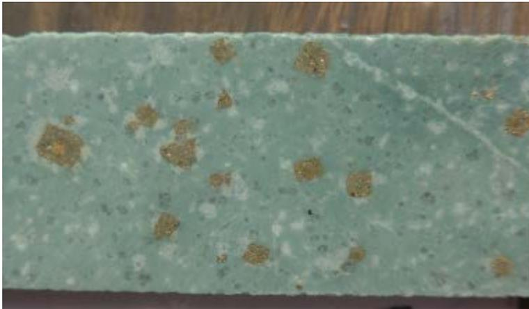
Photo 2. Quartz-eye bearing dacite volcanic with strong chlorite alteration and disseminated cubic pyrite which has replaced mafic minerals from 888.8m in N62DDH015 (Harrington, 2015).
