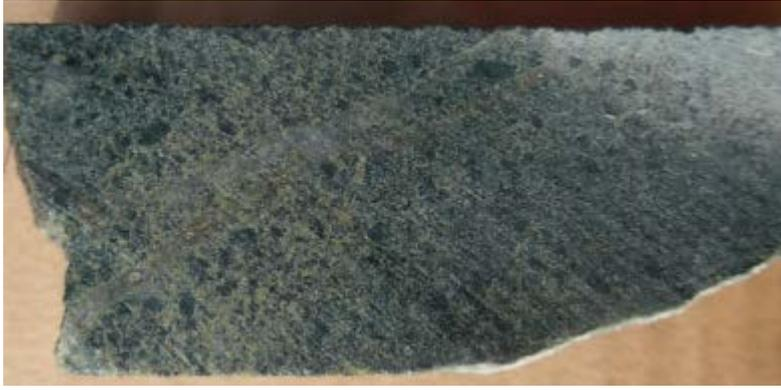
Photo 10. Intense epidote alteration in diorite from 1151.3m in drill hole N62DDH015 (Harrington, 2015).
