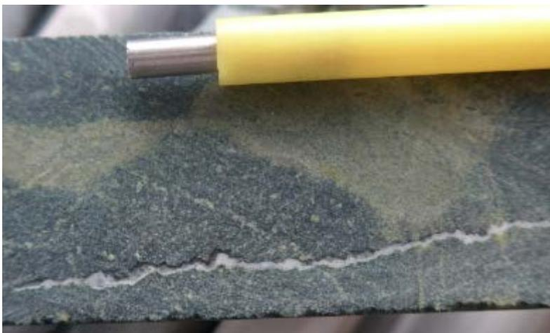
Photo 12. Disseminated magnetite in diorite and on the margins of a thin quartz vein from N62DDH015 (Harrington, 2015).
