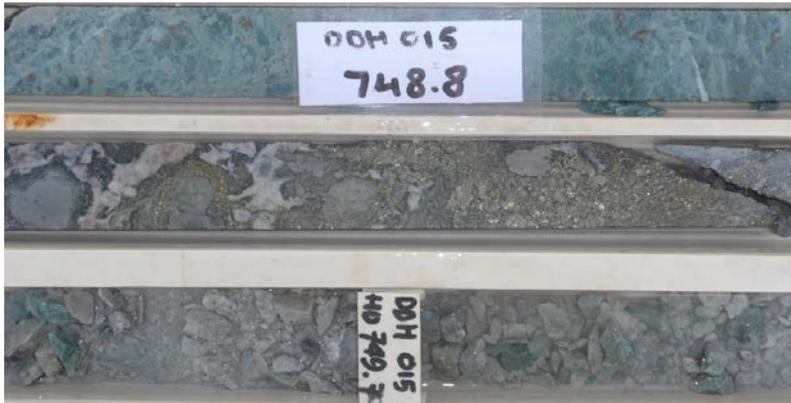
DDH015 748.8m pyrite vein in dacite/silicified fault zone
