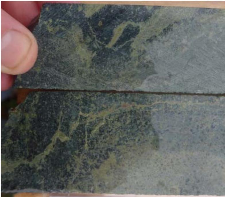
Photo 11. Intense epidote alteration in diorite from 1,179.6m in N62DDH015 (top) and 871.6m in N62DDH012 (bottom) (Harrington, 2015).
