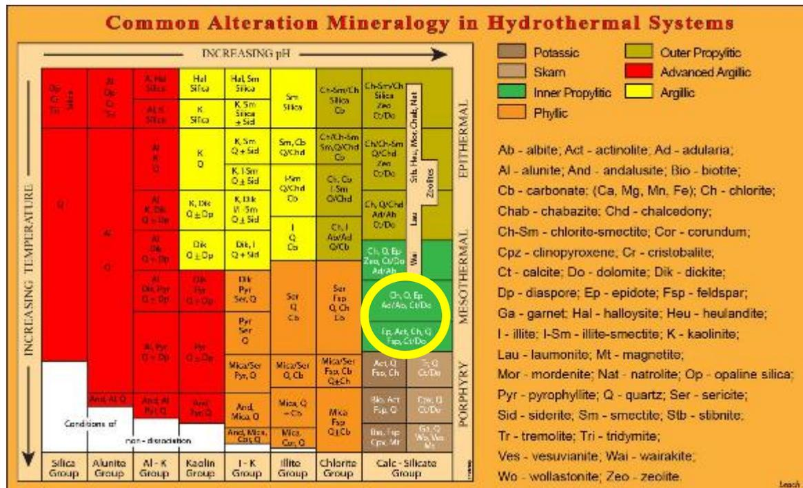
Figure 4. Alteration minerals in hydrothermal systems (Corbett and Leach, 1998) showing the assemblages reported from analysis of Tripela drill core (yellow circle).
