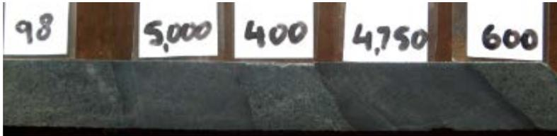
Photo 8. Sub-parallel magnetite-bearing dykes which cuts dacite and has given the core a banded appearance. Magnetic susceptibility values are in CGS units from 144m depth in drill hole N62DDH015 (Harrington, 2015).
