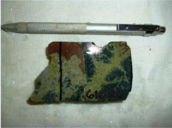
Photo 13. Sample N62PET 61384 which exhibits skarn-like intense epidote-chlorite-quartz-gypsum-calcite-hematite-amphibole alteration of a diorite porphyry from N62DDH012, 863.6m.
