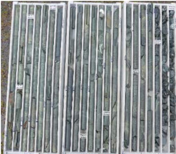
Photo 5. Massive moderate to strongly epidote altered diorite from 1137 to 1156.8m in drill hole N62DDH015. Note a darker magnetic dyke in the middle of the photo from 1143.2 to 1144.1m (Harrington, 2015).
