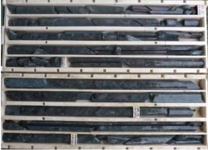
Photo 7. Brecciated diorite with weak epidote alteration from approximately 953-961m in drill hole N62DD015 (Harrington, 2015).
