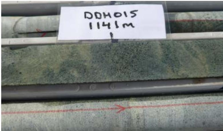
Photo 9. Pervasive epidote alteration in fine grained diorite from 1141m in drill hole N62DDH015 (Harrington, 2015).
