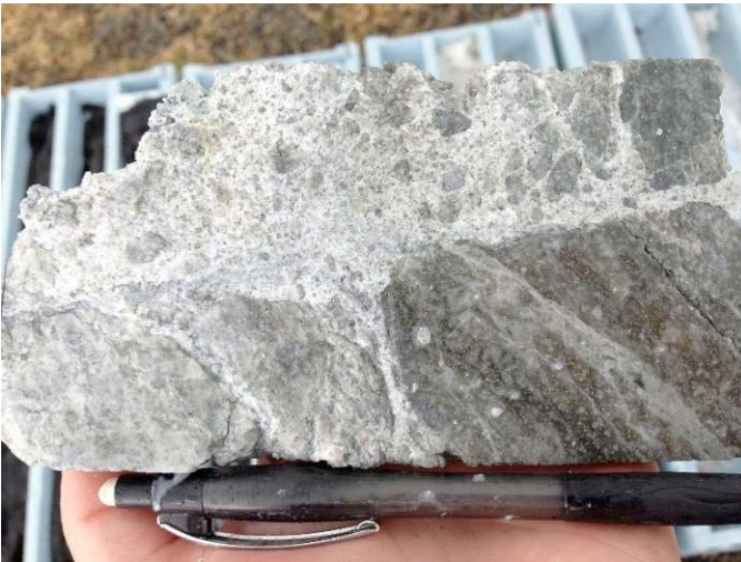
Photo 11. N6DDH001 209.5m clay-pyrite rich brecciated fault zone in silica-sericite altered dacite volcanic.
