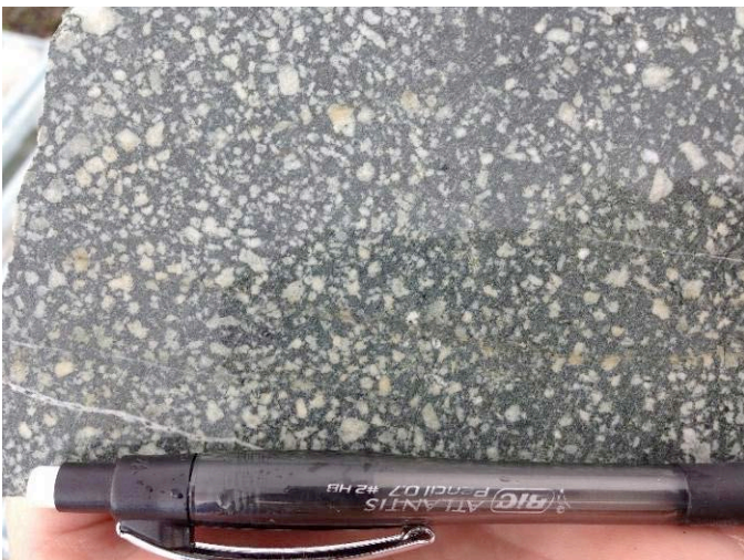
Photo 14. N6DDH001 339m vesiculated and chilled margin of andesite dyke intruding dacite volcanic.
