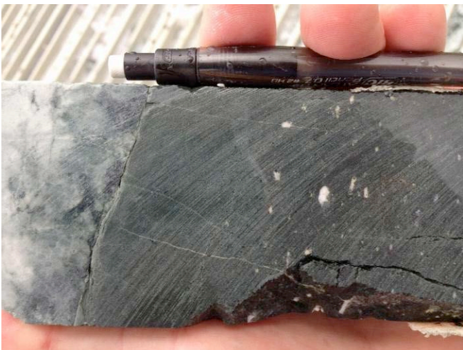
Photo 14. N6DDH001 339m vesiculated and chilled margin of andesite dyke intruding dacite volcanic.
