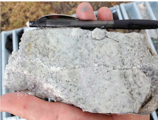
Photo 11. N6DDH001 209.5m clay-pyrite rich brecciated fault zone in silica-sericite altered dacite volcanic.
