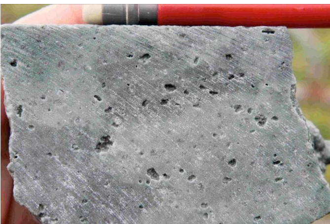
Photo 24. N6DDH002 415.8m showing intense silicification producing pits after hornblende.
