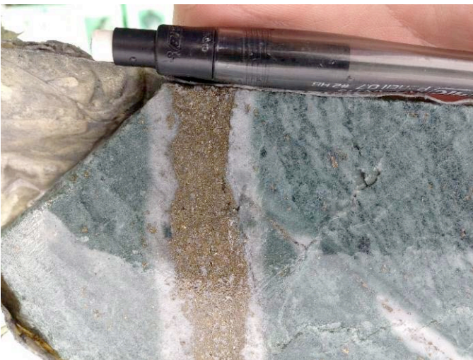
Photo 23. N6DDH001 481m quartz-pyrite D vein with sericite margin
