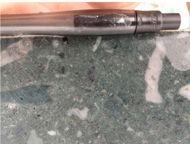
Photo 21. N6DDH001 439.4m polymict matrix supported pebble dyke
