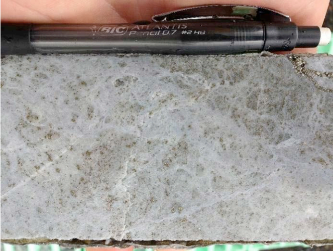
Photo 19. N6DDH001 422m intense silica-sericite stock-work vein
