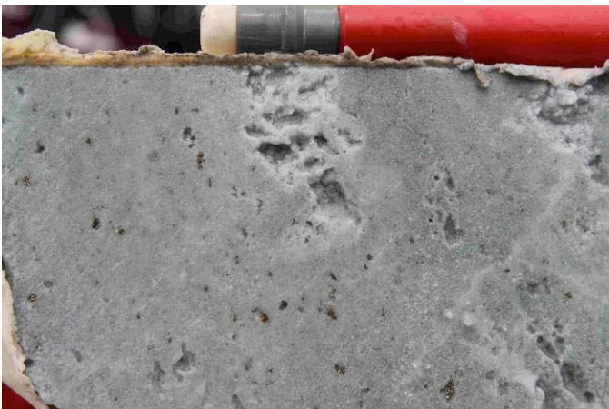
Photo 18. N6DDH001 400.9m intensely silicified dacite volcanic.
